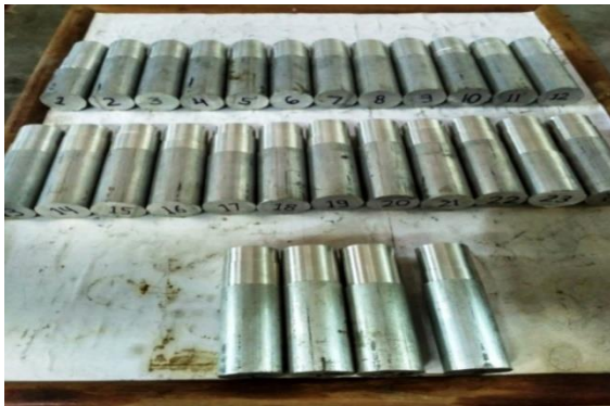
Fig 2: AA6082 Workpiece After Turning
